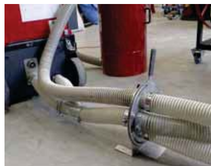
Mobile insertion using switchover function between blowing and suction operation.
